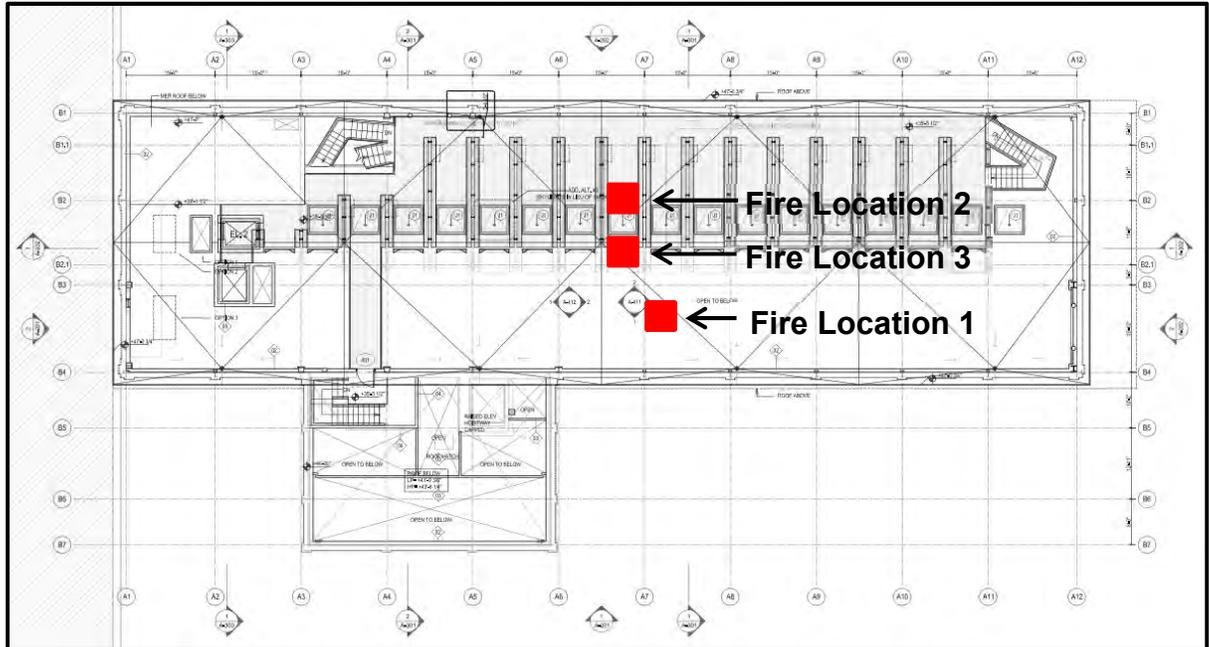
2. Fire Location 2: The fire used in this simulation has been located below the raised second floor, aligned in the center of the stack aisles above it. This type of fire and its location utilize the Design Fire Scenario 2 described above.
