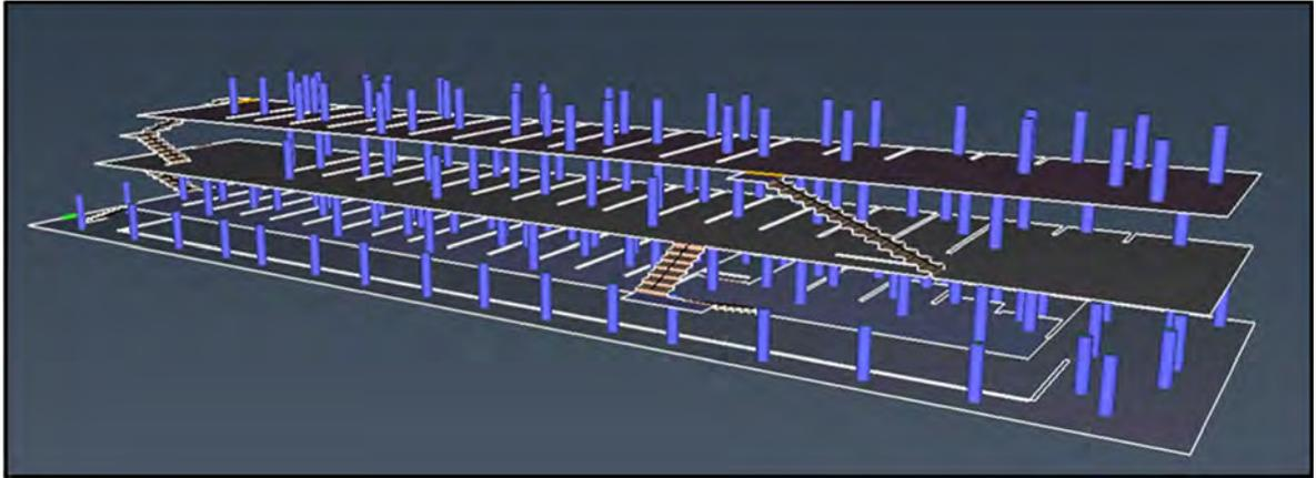
The paths of egress utilized by the occupants within the model are the two stairways located on each end of the raised second floor and the mezzanines/floors above. Once the simulated occupants reach the second floor they proceed to exit the building by either the exit door on the south wall into stair 1 or the exit stair door on the east wall.
