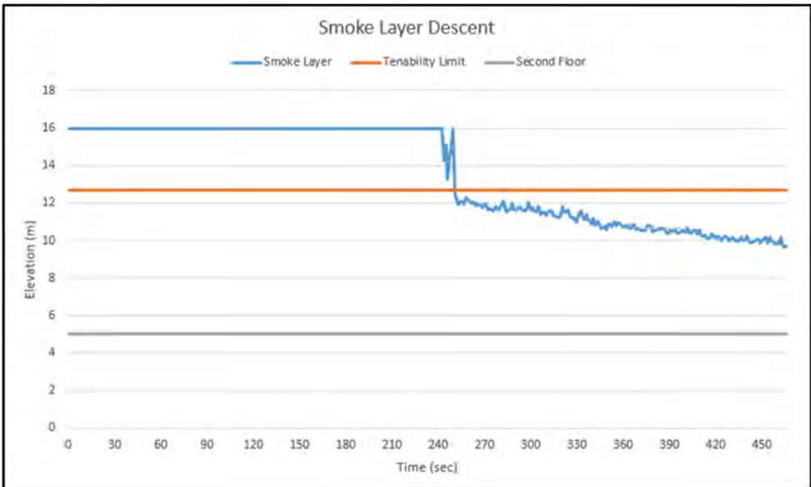
As seen from the graph above, developed from the fire model data, the smoke layer forms enough to begin descending at approximately 240 seconds. Once the smoke layer develops it descends at an average rate of 0.06 meters per second. At approximately 250 seconds it can be observed that the tenability limit for the top floor has been reached thus meaning that evacuation from the top floor must be accomplished before 250 seconds.
